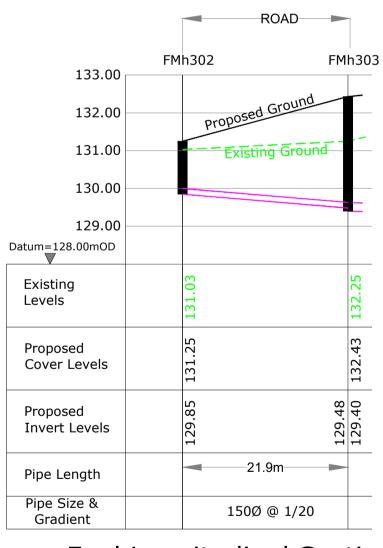
Foul Longitudinal Section FMh302 to FMh303 Vertical Scale 1:100 Horizontal Scale 1:500
